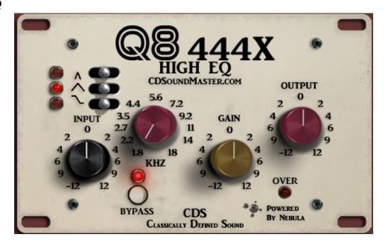
This plug-in allows you to access all three versions of the High EQ filters directly from this one Plug-In instance. Choose the first switch to load the Narrow Band Bell-Shaped EQ. Choose the second switch to load the Wide Band Bell-Shaped EQ. Choose the third switch to load the Shelf EQ.
