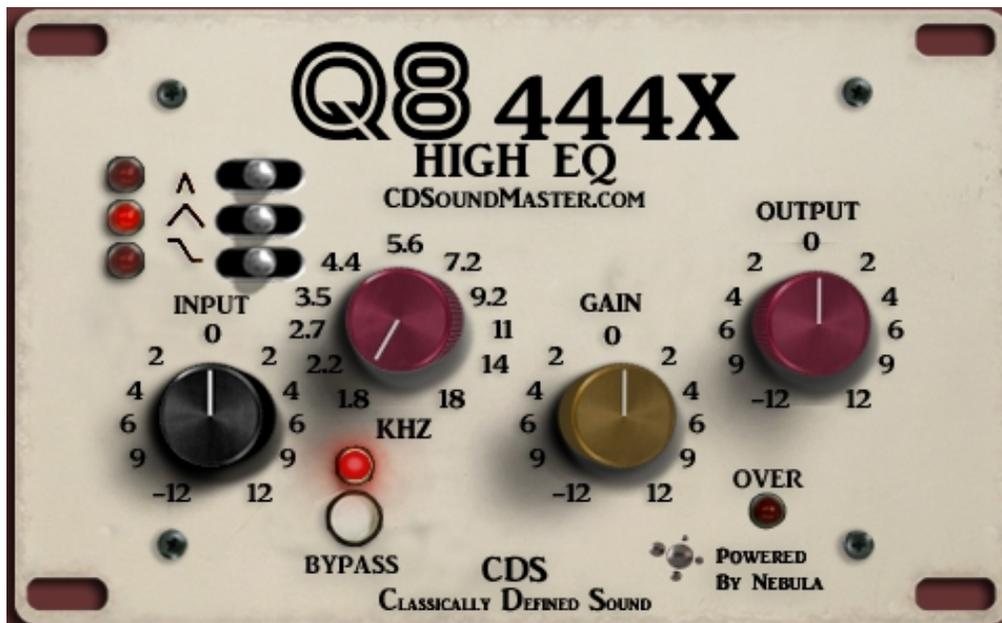
**This plug-in allows you to access all three versions of the High EQ filters directly from this one Plug-In instance. Choose the first switch to load the Narrow Band Bell-Shaped EQ. Choose the second switch to load the Wide Band Bell-Shaped EQ. Choose the third switch to load the Shelf EQ.**
