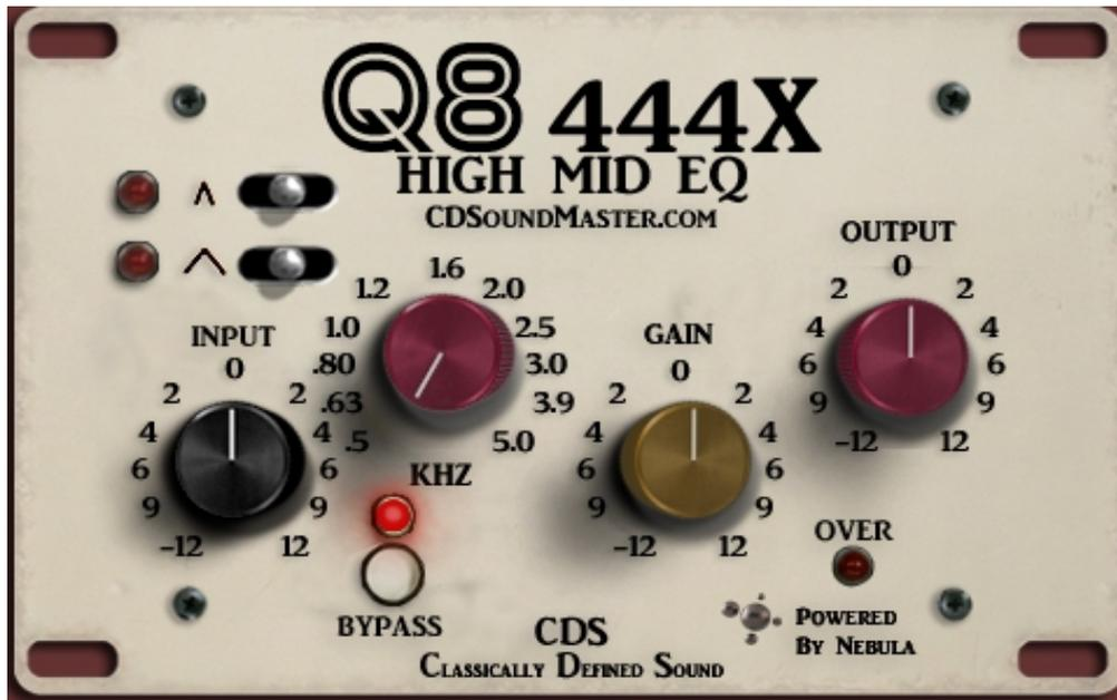
The Mid EQ section of the top-tier Q8 console has two separate controls for two separate frequency ranges: High Mid EQ and Low Mid EQ.
