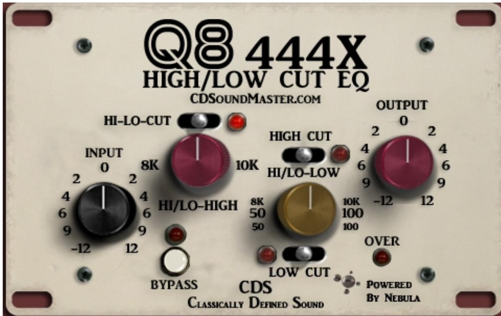
The 'Cut' function of the Q8 is extremely thorough. Not only does it have High Cut and Low Cut, but it has multiple frequency cut-off points for both. To make this entire section of options available from a single user interface, we have made the High/Low Cut EQ module extensive.
